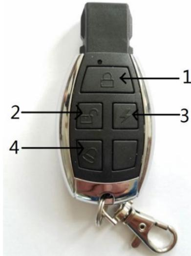
1. "1" is the Alarm Button. when shutting off the main key, pressing one time gently, the horn will ring one loud, the scooter will be on alert. When touching the scooter or driving the scooter, the horn will ring 15 seconds. If forcing to move the scooter, the horn will ring continuously.
